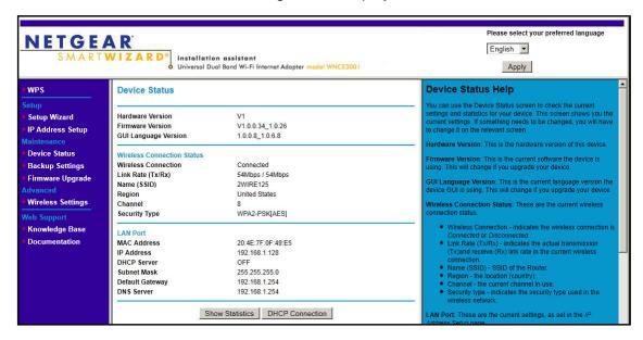
The Device Status screen shows what the current settings are for the Internet adapter. A menu in the left pane allows you to view or change the settings.
